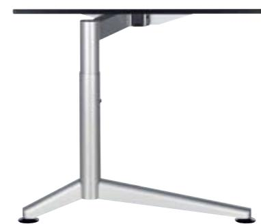
C-frame Positioning range: 62-86 cm adjustable in increments of 2 cm with an Allen key or head screw
